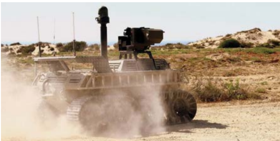
The AvantGuard Mk I is controlled by mobile or portable operational control unit. It can also operate in follow-me mode, where it autonomously trails a dismounted guiding soldier or vehicle. (Photo: G-NIUS)
