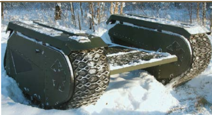
Milrem's tracked UGV platform, pictured above during recent cold-weather trials, is designed to accommodate a range of different payloads, which could include remote weapon systems. (Photo: Milrem)
